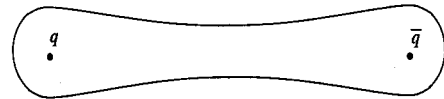
Figure 1. Experiment and computer simulations indicate that if one separates a quark and anti-quark (labeled q and \bar{q} in the figure) by a relatively large distance R , a little-understood ‘colour electric flux tube’ forms between them. As a result, the energy grows in proportion to R .
