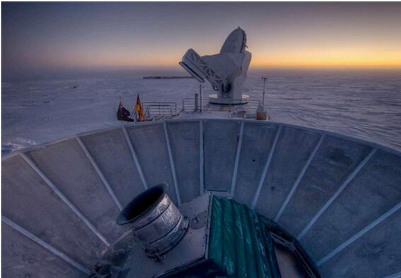
Telescope as compact as possible while still having the angular resolution to observe degree-scale features.
